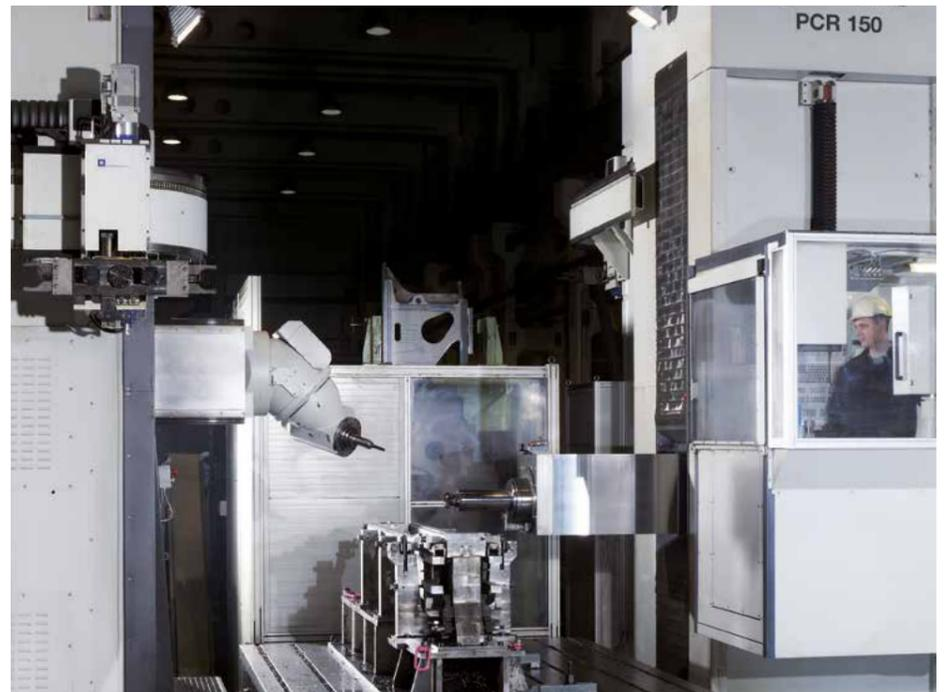
Duo arrangement: coupled machining of a workpiece from two sides on the floor plate
