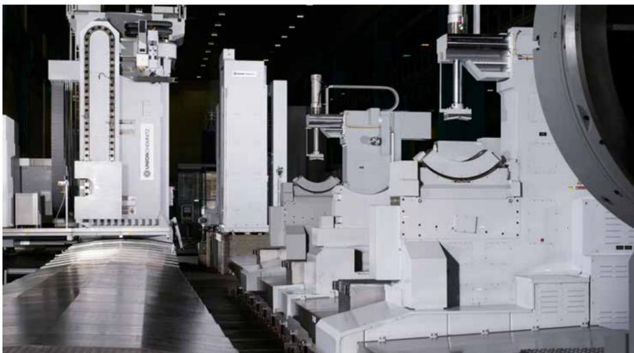
The new rotor slotter: a combination of a PCR 260 (left) and a set-up system by WaldrichSiegen
